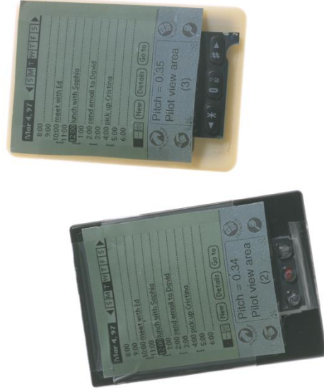
Prototypes Used for Button Location and Feel Experiments
