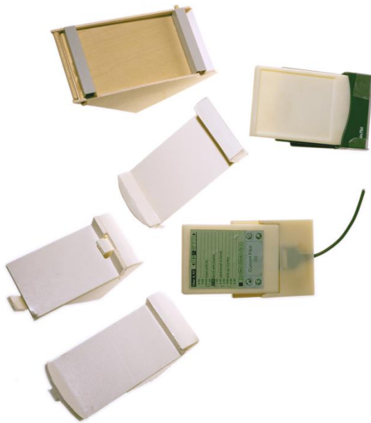
Foam, Wood and Mechanical Prototypes of HotSync Cradle
