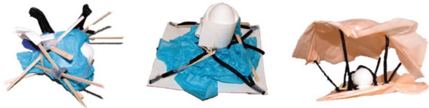
Fig. 9 Left: Participant 3 (iteration) successfully protected the egg at 5 ft. Middle: Participant 18 (iteration) protected at 2 ft. Right: Participant 28 (iteration) protected the egg only at 1 ft
