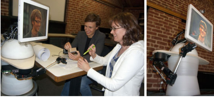
Fig. 6 A robotic avatar at work. On the left is a robotic avatar in use during a design session. On the right is a closer view of its remotely controlled components. The remote participant who operates the robot uses onscreen buttons to make pre-programmed movements, such as “wave” or “point near emphatically,” with its arm, and a handheld gesture-based controller to make front-to-back, left-to-right and tip-up or tip-down motions with its head, which includes a video screen, camera and microphone
