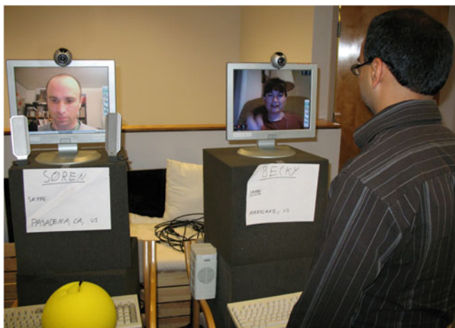
Fig. 3 Early physical avatars. This image shows two distant participants speaking with a local moderator by video chat. Their screen images are positioned atop kiosks at eye-level, and each has a personal camera, microphone and speaker for close-up conversation. Their names, location in the world, and instant messaging identity are shown so local participants can join them in the back-channel chat. A foam microphone ball, passed around by local speakers during Q&A dialog, is visible at the bottom left
