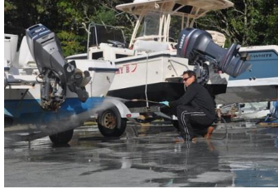
Pressure washing the hull
