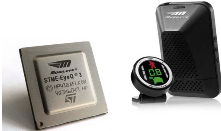
Exhibit 4 Mobileye's EyeQ Chip for OEMs and Mobileye's Camera Module (which attaches behind a car's rearview mirror) and Alert Display for the Aftermarket
